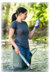
Choose from several field-ready sensors. The selected sensor set will determine the diameter of the TROLL 9500—sub-2 inch or sub-4 inch.
